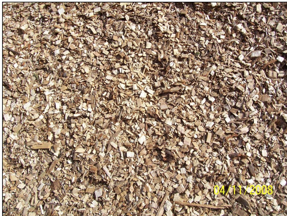
Figure 2. Bole Chips for Use in a Biomass Thermal Application.
